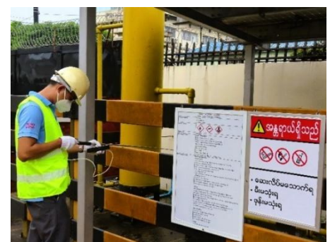
Gas Leakage Test
